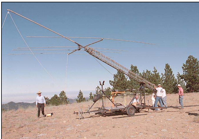
15-meter beam goes up with Warren Dowler's new horizontal-seeking beam mount, on the rebuilt tower trailer fitted with a "new" Tri-Ex three-section tower
