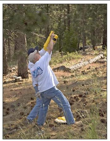
Pneumatic Long Wire Antenna Launcher
