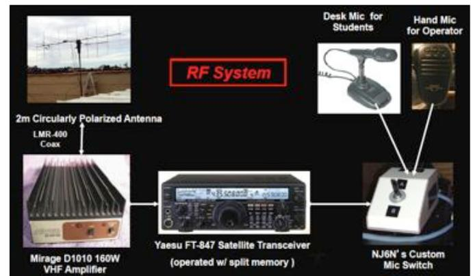
**Figure 7: Primary RF System used for the ARISS contact.**
