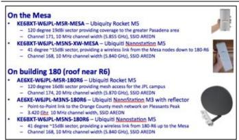
Figure 2: Test Mesh network setup at JPL to support the October Guest Speaker.
