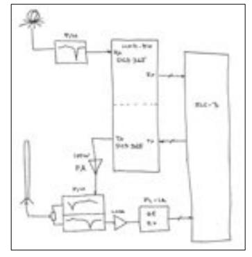
Figure 5: Proposed 445.20 repeater re-configuration
