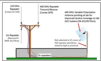
Figure 4: Proposed repeater antenna installation
