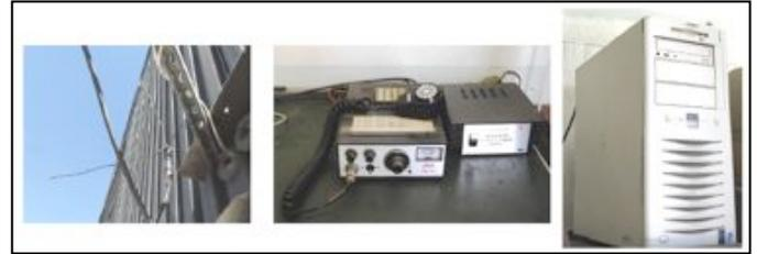
**Figure 3: Current JPL IRLP/Echolink Node in 180-R6. Simple 220 MHz ground plane antenna (left), Clegg FM-76 transceiver (center) and PC running Linux & the IRLP application (right)**
