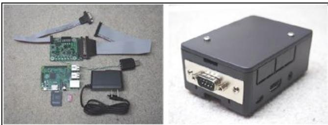
**Figure 2: PiRLP kit (left) and prepackaged unit (right)**
