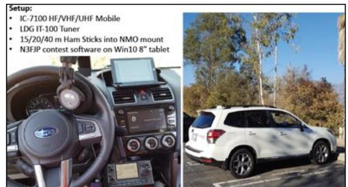
Figure 3: KF6RTB mobile HF installation
