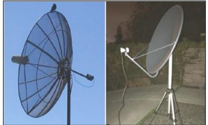
**Figure 6: C band antenna (left) and KB3UUS's (\$100 on eBay) Ku band antenna (right)**
